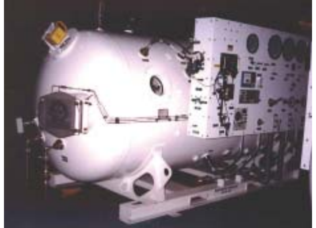
Standard Navy Double Lock Chamber (SNDL).
