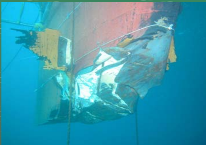
Damage to bottom of rudder.
