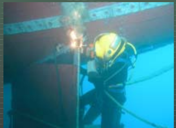
USS EMORY S. LAND Diver burning top of rudder to increase clearance from hull.
