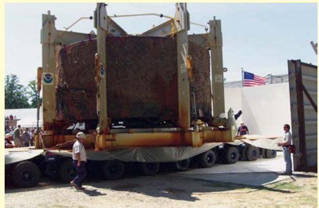
The USS MONITOR's Revolving Gun Turret is driven into the awaiting conservation tank after being delivered to the Mariners' Museum in August of 2002.
