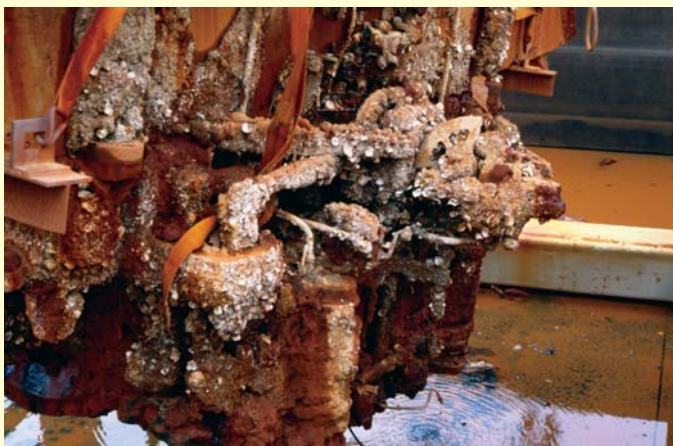
For almost 140 years the 30-ton side lever steam engine that propelled the historic ironclad USS MONITOR has been resting in its watery grave 240 feet below sea-level, 16 miles off the coast of Cape Hatteras. The engine is now undergoing restoration and visitors can watch conservators slowly remove over a century of corrosion from this historic propulsion system.
