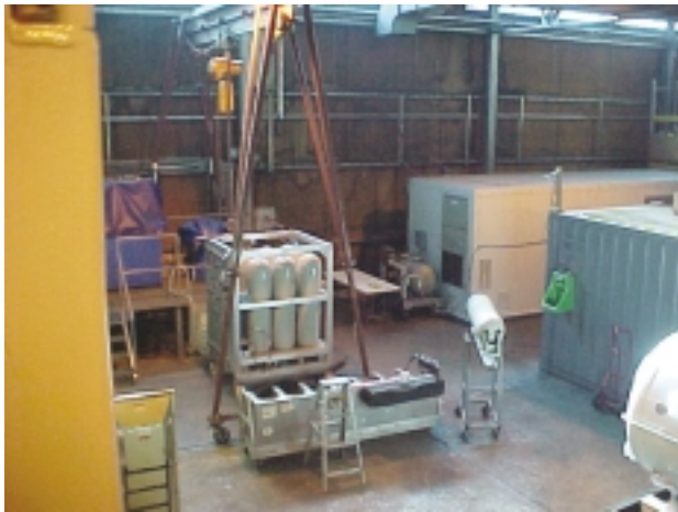
FADS III flasks being hydrostatic tested.
