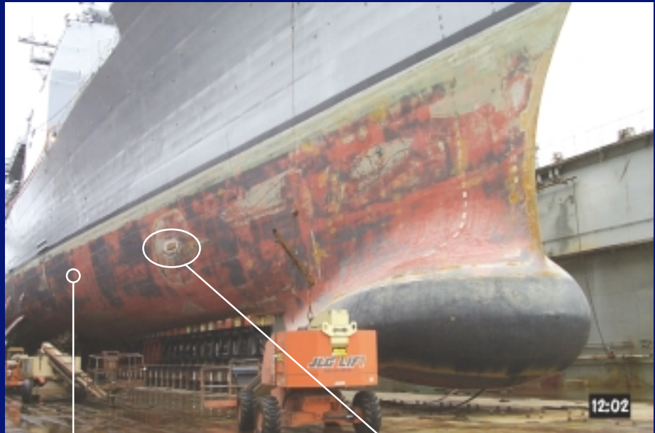
Forward 4-foot long anode and dielectric shield.
