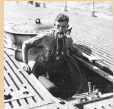
Crewman A.L. Rosenkotter of USS V-5 (SC 1) demonstrates the use of the submarine's after escape hatch and the emergency escape "lung" during V-5's trials in July of 1930.
