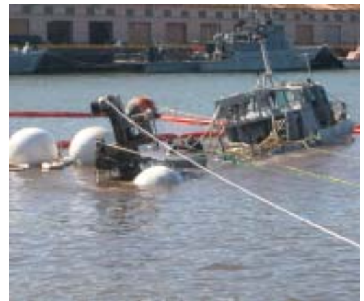
After putting in internal flotation devices and with the amount of sand retained while aground on rocks, more external flotation devices were required for the port aft corner.
